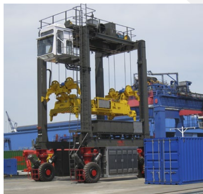
E-Straddle Carrier with Battery Charging Systems
